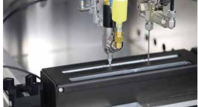
Brush and blowout station ProtectoXC
