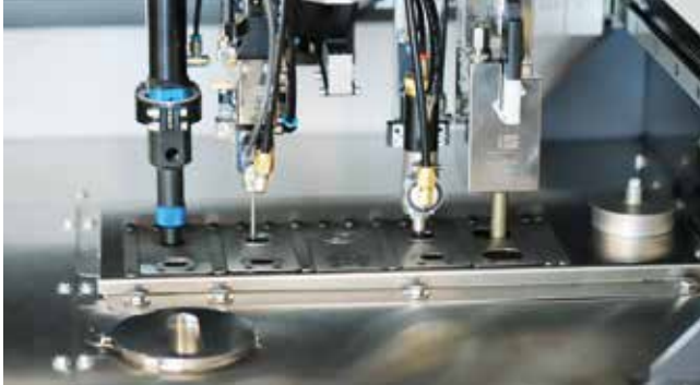
Brush and blowout station ProtectoXP
