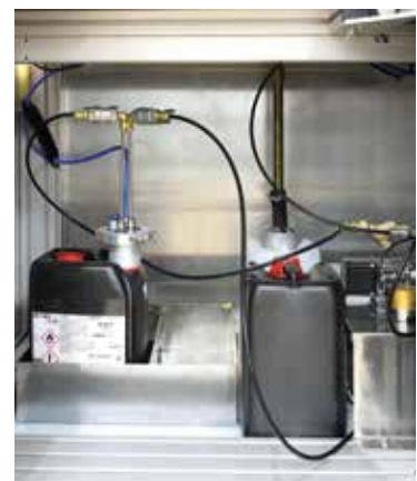
Lacquer supply at the front of the plant (XC)
