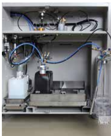
Easily accessible lacquer supply at the back of the plant (XP)
