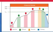
A defined quantity of an inert fluid (usually perfluorpolyether) is vaporized during reflow soldering in the process chamber, which is hermetically sealed by means of a bulkhead. The vapor allows for extremely effective heat transfer to the PCBs due to the release of heat during condensation, and the temperature of the medium remains constant. In addition to this, the medium's boiling point limits the
