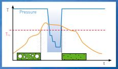
Void-free soldering with lead-free solders is an important prerequisite for the production of power electronics. However, minimal void rates are only possible with soldering processes which subject the molten solder to a vacuum, making it easier for any remaining residues to escape from the solder joints. For this reason, the Condenso can be equipped with a vacuum pump upon request. This results in solder joints with surface contact ratios of greater than 99% in many cases.
